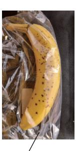
Bananas placed in LDPE bags containing our apatite-coated titanium dioxideblended at 1% concentrationshowed no deterioration whatsoever from their original state.
